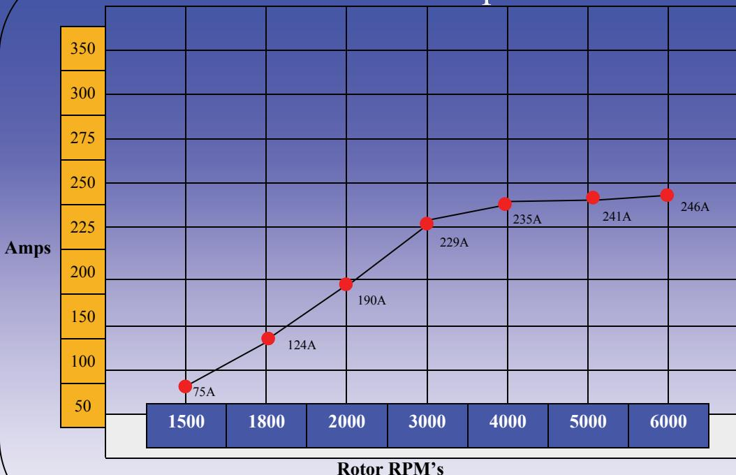
Alternators are tested at 13.5 Volts
